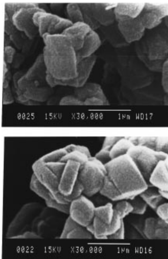
Figure 14. Scanning electron micrographs for ZCVD850 (top) and ZCVD850 oxidized at 50% burnoff (bottom).
